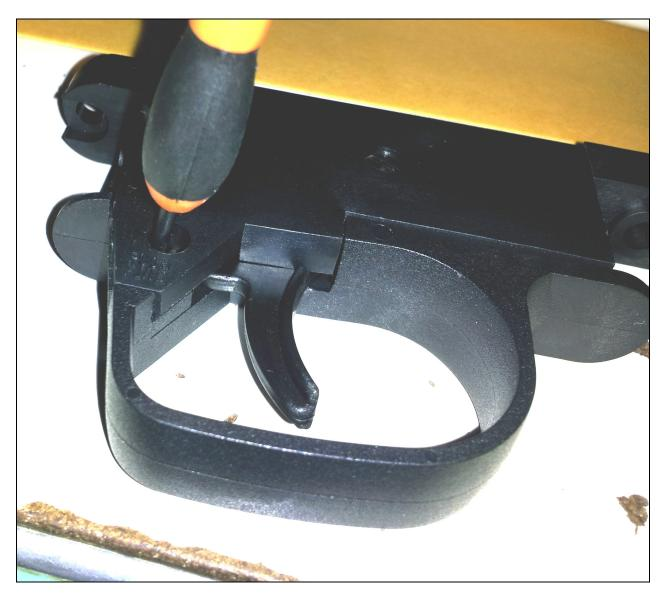
Push spring forward until the tip is exposed directly behind the trigger.
