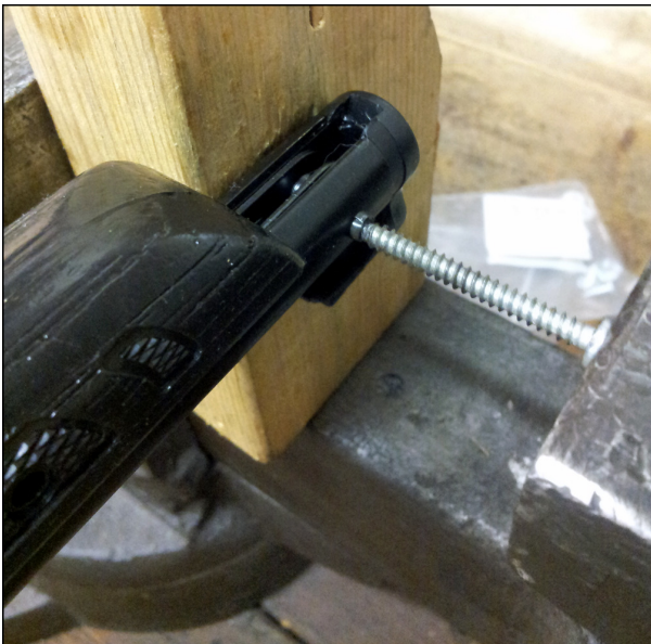
Again, this shows me working on the pump lever pin, but the process for driving out the forearm pins is the same. Close the vise jaw against the screw to drive out the pin. Reverse the process for driving the pins in.
