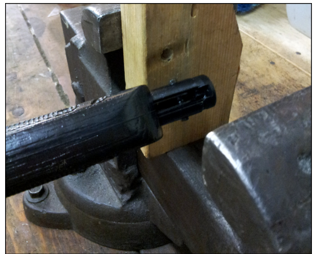
This photo shows me working on the pump lever roll pin, but the process is the same for the forearm roll pins. Situate the gun so that the pins drive into the hole you've drilled.
