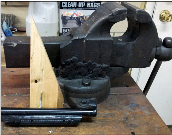
A bench vise, piece of wood with hole drilled into it and an appropriately sized screw or nail will drive the pins out and back in.
